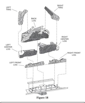
Warning: Failure to position the parts in accordance with this diagram or failure to use only parts specifically approved with this appliance may result in property damage or personal injury.
